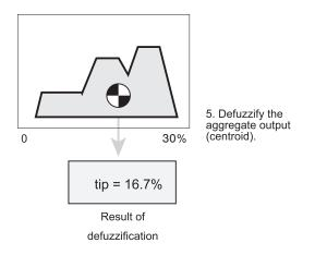
While the aggregate output fuzzy set has covers a range from 0% though 30%, the defuzzified value is between 5% and 25%. These limits correspond to the centroids of the cheap and generous membership functions respectively.
