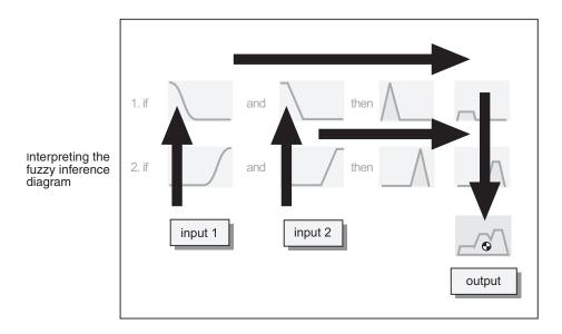
In this figure, the flow proceeds up from the inputs in the lower left, then across each row, or rule, and then down the rule outputs to finish in the lower right. This compact flow shows everything at once, from linguistic variable fuzzification all the way through defuzzification of the aggregate output.
