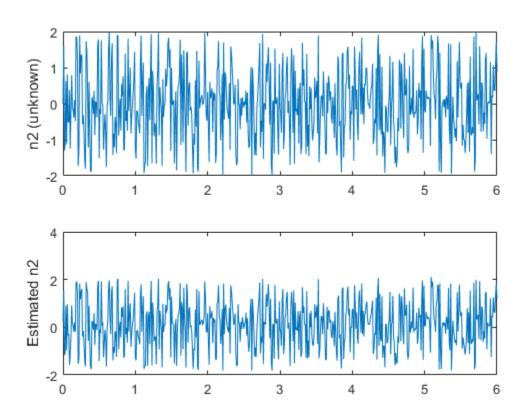
The estimated information signal is equal to the difference between the measured signal, m, and the estimated interference (ANFIS output).
