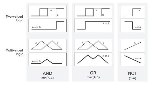
Given these three functions, you can resolve any construction using fuzzy sets and the fuzzy logical operation AND, OR, and NOT.
