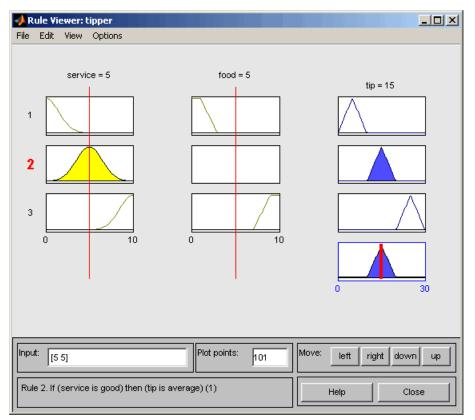
The Rule Viewer displays a roadmap of the whole fuzzy inference process. It is based on the fuzzy inference diagram described in the previous section. You see a single figure window with 10 plots nested in it. The three plots across the top of the figure represent the antecedent and consequent of the first rule. Each rule is a row of plots, and each column is a variable. The rule numbers are displayed on the left of each row. You can click on a rule number to view the rule in the status line.
