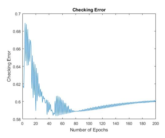
The plot shows that the smallest value of the validation data error occurs at the 52nd epoch, after which it increases slightly even as anfis continues to minimize the error against the training data all the way to the 200th epoch. Depending on the specified error tolerance, the plot also indicates the ability of the model to generalize the test data.
