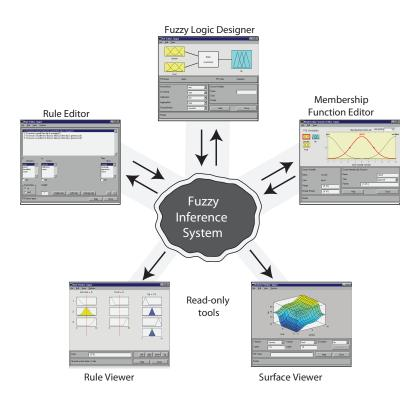
The following figure shows how the main components of a FIS and the three editors fit together. The two viewers examine the behavior of the entire system.
