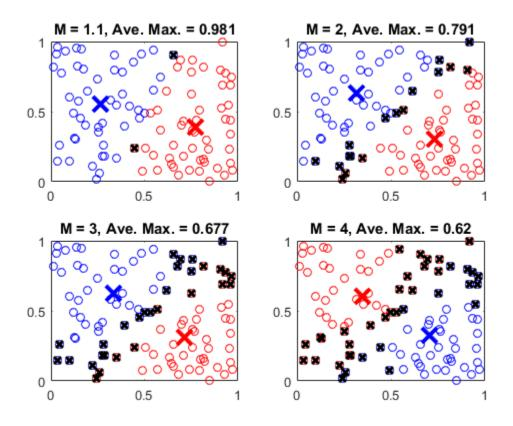
A given data point is classified into the cluster for which it has the highest membership value, as indicated by maxU. A maximum membership value of 0.5 indicates that the point belongs to both clusters equally. The data points marked with a black **x** have maximum membership values below 0.6. These points have a greater degree of uncertainty in their cluster membership.
