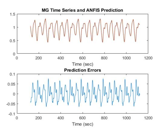
The difference between the original MG time series and the values estimated using anfis is very small. Therefore, you can only see one curve in the first plot. The
