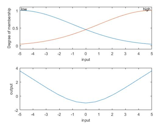
As this example shows, Sugeno-type system gives you the freedom to incorporate linear systems into your fuzzy systems. By extension, you could build a fuzzy system that switches between several optimal linear controllers as a highly nonlinear system moves around in its operating space.
