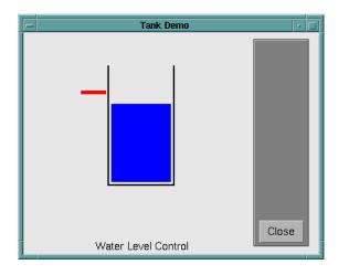
A controller for the water level in the tank needs to know the current water level and it needs to be able to set the valve. Your controller's input is the water level error (desired water level minus actual water level), and its output is the rate at which the valve is opening or closing. A first pass at writing a fuzzy controller for this system might be the following:
