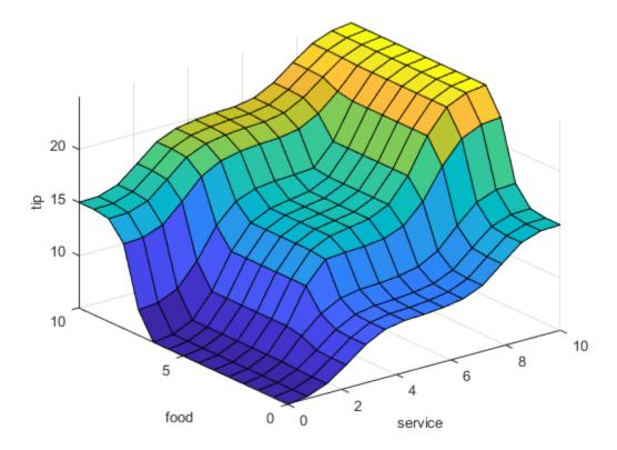
This plot was generated by the three rules that accounted for both service and food factors. The mechanics of how fuzzy inference works is explained in the Overview section of Foundations of Fuzzy Logic topic. In the topic, Build Mamdani Systems (GUI), the entire tipping problem is worked through using the Fuzzy Logic Toolbox (TM) apps.
