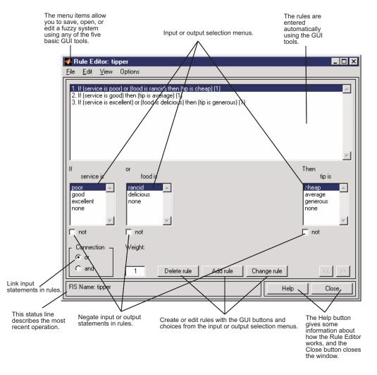
Constructing rules using the graphical Rule Editor interface is fairly self evident. Based on the descriptions of the input and output variables defined with the **Fuzzy Logic Designer**, the Rule Editor allows you to construct the rule statements automatically. You can:
