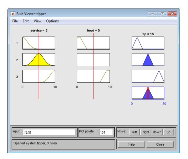
ruleview(fis) opens the Rule Viewer for the fuzzy inference system, fis. It is used to view the entire implication process from beginning to end. You can move around the line indices that correspond to the inputs and then watch the system readjust and compute the new output. Refer to "The Rule Viewer" on page 2-50 for more information about how to use ruleview.
