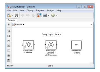
The Fuzzy Logic Toolbox library contains the Fuzzy Logic Controller and Fuzzy Logic Controller with Rule Viewer blocks. It also includes a Membership Functions sublibrary that contains Simulink blocks for the built-in membership functions.
