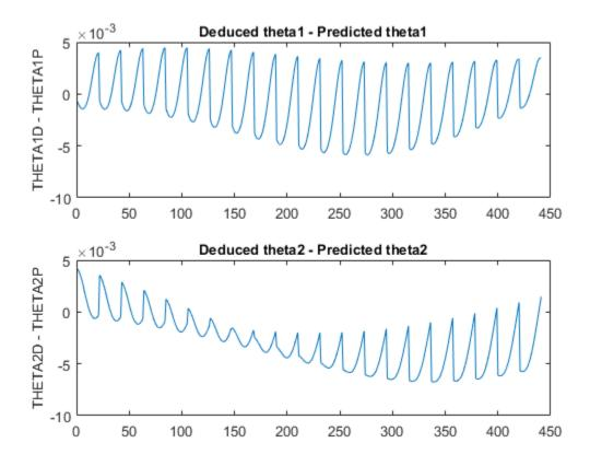
The errors are in the 1e-3 range which is a fairly good number for the application it is being used in. However this may not be acceptable for another application, in which case the parameters to the anfis function may be tweaked until an acceptable solution is arrived at. Also, other techniques like input selection and alternate ways to model the problem may be explored.
