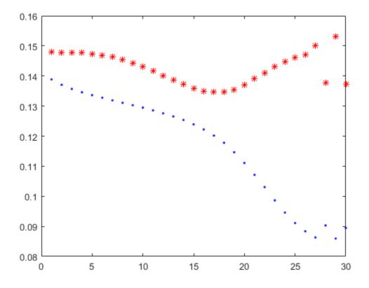
The minimum validation error occurs at epoch 17. The increase in validation error after this point indicates overfitting of the model parameters to the training data. Therefore, the tuned FIS at epoch 17, chkFIS, exhibits the best generalization performance.
