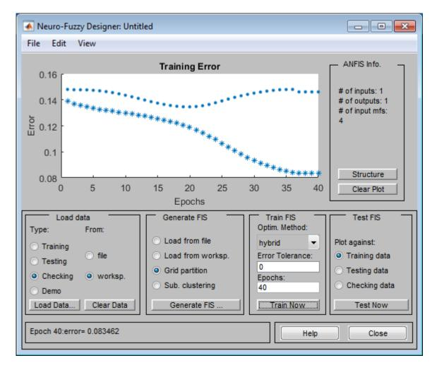
The plot shows the checking error as  $\blacklozenge \diamondsuit$  on the top. The training error appears as  $\ast \ast$  on the bottom. The checking error decreases up to a certain point in the training, and then it increases. This increase represents the point of model overfitting. anfis chooses the model parameters associated with the minimum checking error (just prior to this jump point). This example shows why the checking data option of anfis is useful.
