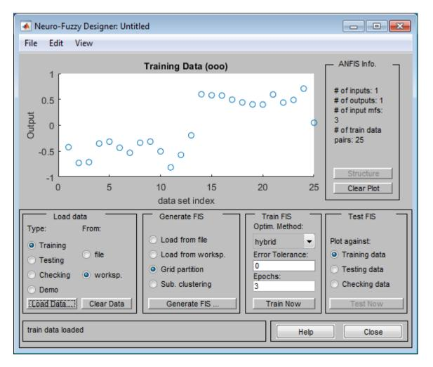
The horizontal axis is marked **data set index**. This index indicates the row from which that input data value was obtained (whether or not the input is a vector or a scalar).
