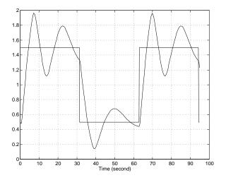
You need to add another input, the water level's rate of change, to slow down the valve movement when it gets close to the right level.
