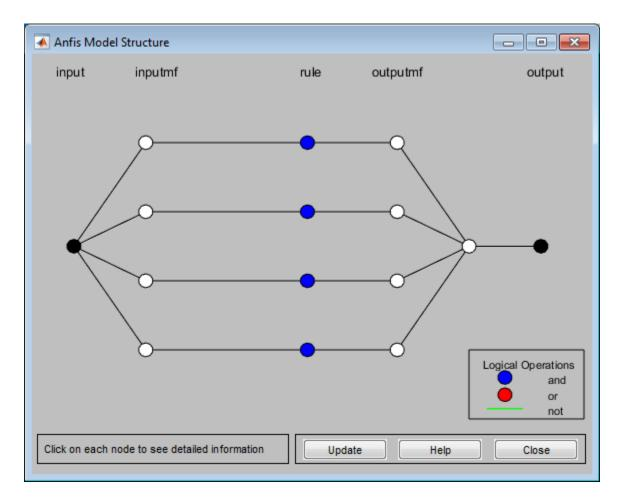
The branches in this graph are color coded. Color coding of branches characterize the rules and indicate whether or not *and*, *not*, or *or* are used in the rules. The input is represented by the left-most node and the output by the right-most node. The node represents a normalization factor for the rules. Clicking on the nodes indicates information about the structure.
