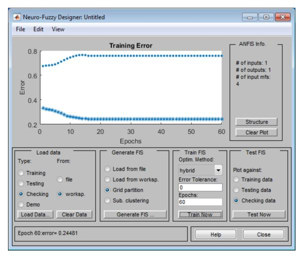
In this case, the checking error is quite large. It appears that the minimum checking error occurs within the first epoch. Using the checking data option with anfis automatically sets the FIS parameters to be those associated with the minimum checking error. Clearly this set of membership functions is not the best choice for modeling the training data.
