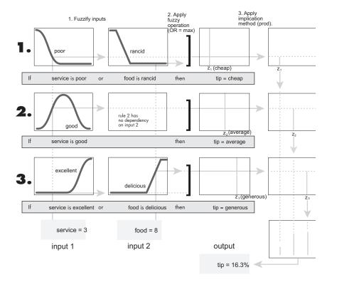
The preceding figure shows the fuzzy tipping model developed in previous sections of this manual adapted for use as a Sugeno system. Fortunately, it is frequently the case that singleton output functions are sufficient for the needs of a given problem. As an example, the system tippersg.fis is the Sugeno-type representation of the now-familiar tipping model. If you load the system and plot its output surface, you see that it is almost the same as the Mamdani system you have previously seen.
