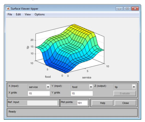
The Surface Viewer is a graphical interface that lets you examine the output surface of an FIS for any one or two inputs. You can examine an FIS that is:
