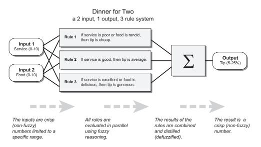
Information flows from left to right, from two inputs to a single output. The parallel nature of the rules is one of the more important aspects of fuzzy logic systems. Instead of sharp switching between modes based on breakpoints, logic flows smoothly from regions where the system's behavior is dominated by either one rule or another.
